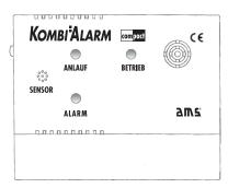
The system is fitted out with the 3 following LED displays:
